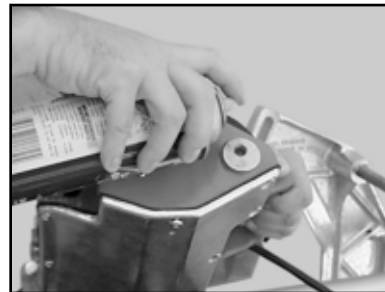
(N) Lubricate the Cutting Head Adjustment Knob retaining holes
