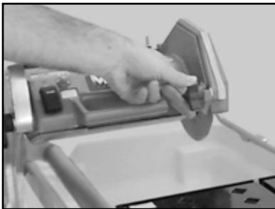
(G) Close the Outer Blade Guard and tighten the Blade Guard Retaining Screw
