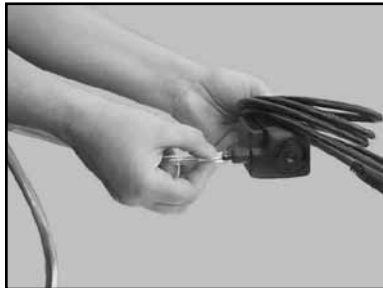
(D) Remove the Transfer Tube and check flow. If flow exists, go to Step F
