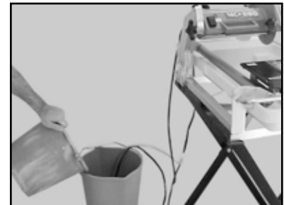
(C) Fill the external container until water completely covers the Water Pump suction
