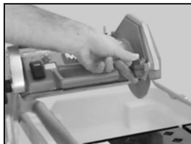
(H) Close the Outer Blade Guard and tighten the Blade Guard Retaining Screw
