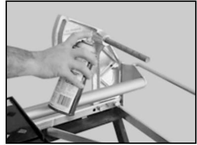
(L) Lubricate the Cutting Head Pivot Shaft
