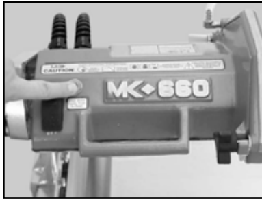
(A) Allow motor to cool and depress motor Overload Reset Switch
