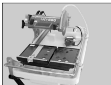
(B) Place the Water Pump in the back of the Water Pan
