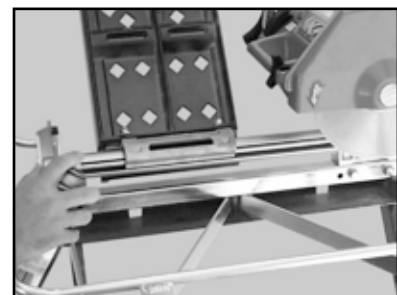
(C) Lubricate the Guide Bar
