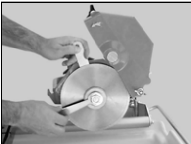
(G) Install the Retaining Nut and Outer Flange. Hold the Shaft using the Inner Flange Retaining Wrench and tighten using the Blade Wrench
