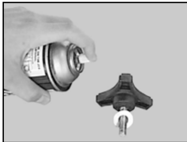
(M) Lubricate the Cutting Head Adjustment Knob
