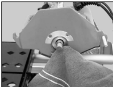
(E) Clean around the Motor Shaft and clean the Inner Flange
