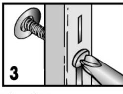
Using #2 Phillips, press tip of E-Z Ancor<sup>®</sup> into drywall.
