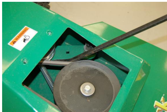
Removing tension on the blade belt
